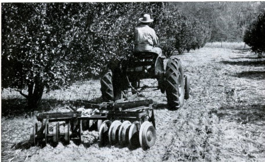
Farmall-A tractor pulls a No. 10-A, specially equipped with automatic angling device and depth gauges.
