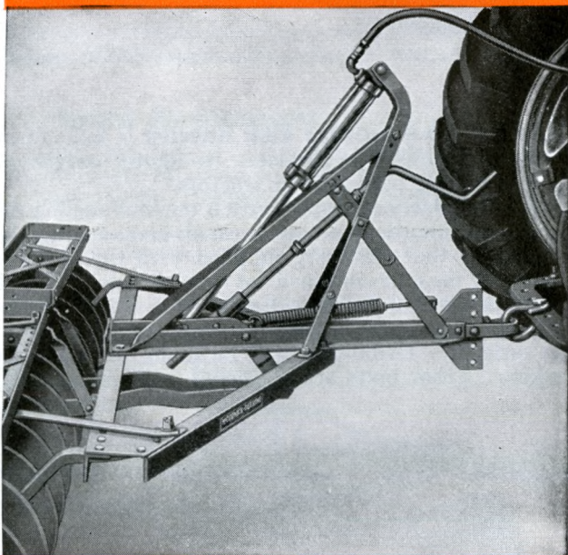
Detail of hydraulic de-angling unit for use with No. 10-A harrows equipped with manual-set (screw-type) gang angling. Nos. 9 and 7 series harrows with manual-set gang angling (special) can be provided with similar equipment.
