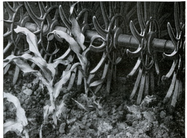
Most weeds get their start near the surface. By using the rotary hoe as soon as the weeds begin to sprout, such weeds are easily dislodged and exposed to the sun.
