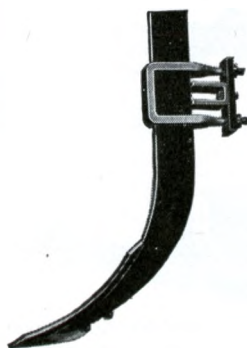
Detail of special light No. 1 subsoil attachment.
