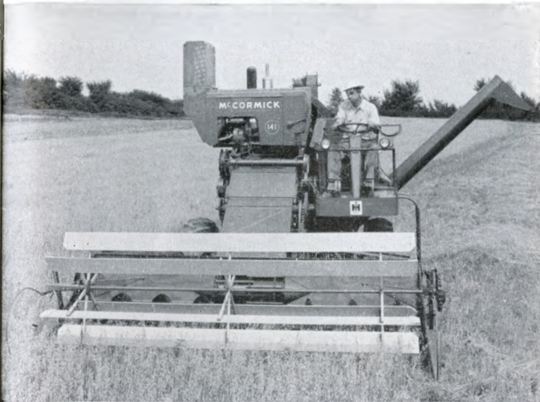
BIG No. 141 SELF-PROPELLED makes quick work of large-acreage harvests. IH variable-speed propulsion drive lets you pick any one of an uncalculated number of travel speeds—and change on the go. You raise 10, 12, or 14-foot platform hydraulically . . . empty 50-bushel grain tank without stopping. IH 64-hp engine insures sure, steady power for the toughest going.
