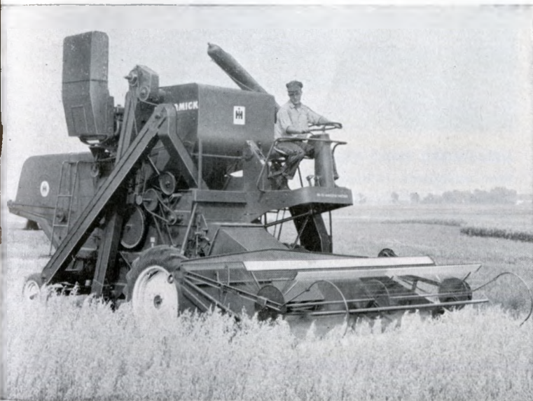
No. 101 SELF-PROPELLED is a new 10-foot Harvester-Thresher with every modern feature. The operator's platform is high up out of the dust for comfortable operation through its three gears .96 to 13 mph speed range. Hydraulically controlled to cut from the ground up to 33 inches, the big 28-inch cylinder and separator give the No. 101 extra capacity to save more clean grain per acre for you.
