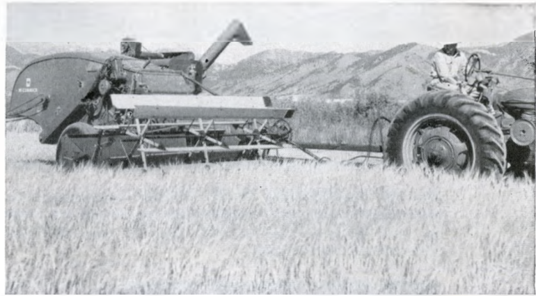
BIG No. 140 PULL-TYPE has a 9-foot hydraulically controlled pickup platform, or a 9-foot platform with a three-foot extension for direct cutting of a full 12-foot swath. Gives you capacity and performance advantages of No. 141 to clean-thresh windrows from as large as 15-foot swath. Grain tank has 45-bushel capacity, and you have a choice of engine or pto drive.
