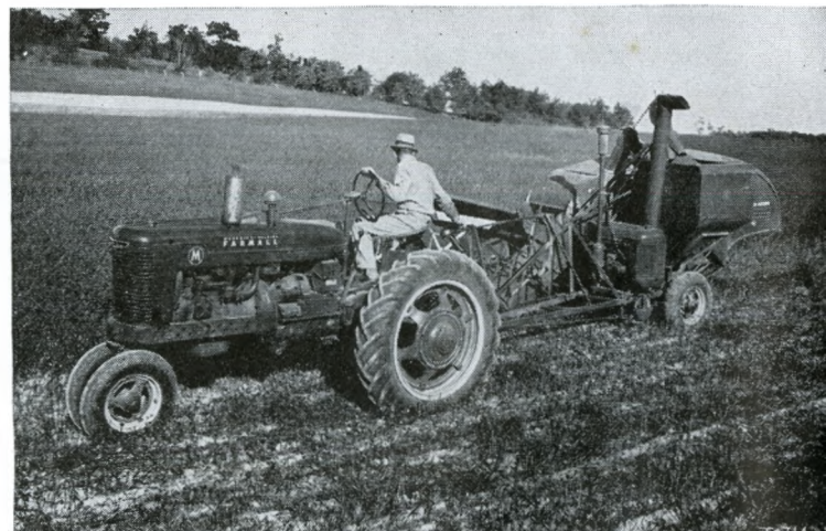
Adjustments for operating the No. 62 combine are convenient for one-man control. This machine is combining flax.
